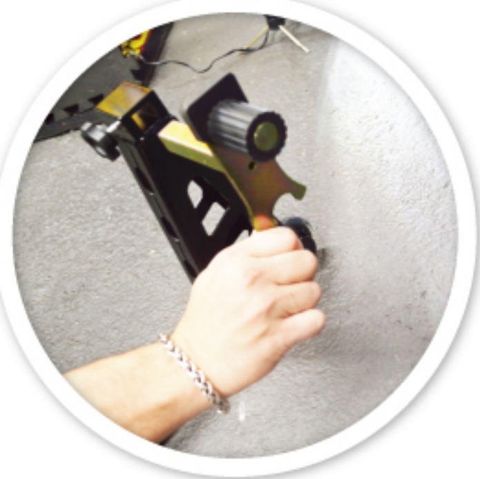
Swingarm Paddle Lift (Ensure Rear Swingarms are Flat and Even on both sides before lifting)
